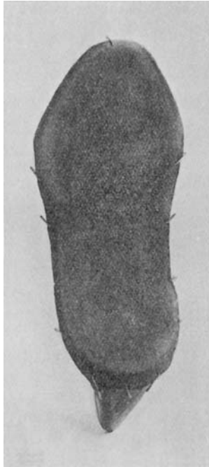
Fig. 17. INNERSOLE BLOCKED TO THE LAST
