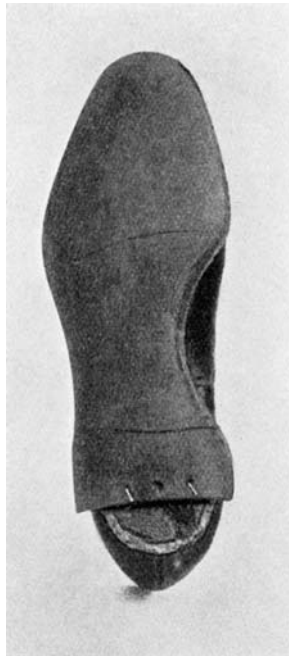
Fig. 63. SOLE ROUNDED AND CHANNEL MARKED
