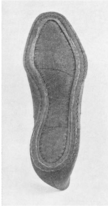
Fig. 55. SEAM TRIMMED AND WELT ROUNDED
