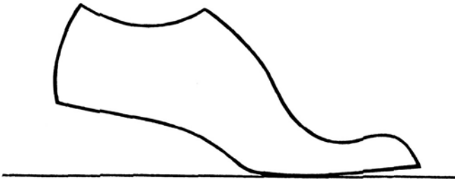
FIG. 36. DIAGRAM SHOWING LAST WITH DROP WAIST
