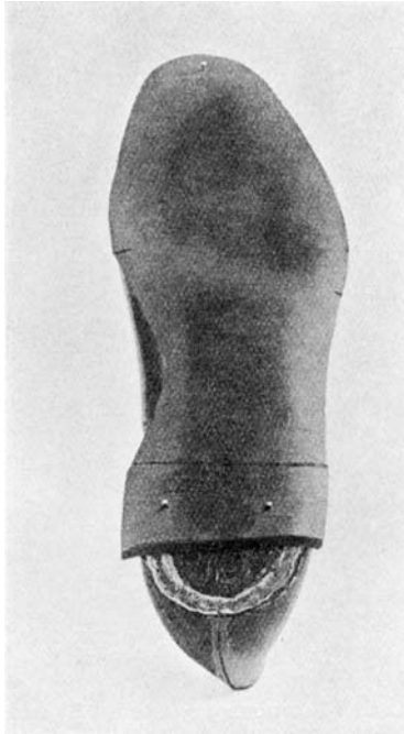
Fig. 60. SOLE FITTED FOR ROUNDING
