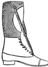
FIG. 42. SIMPLE DROP FOOT APPLIANCE
