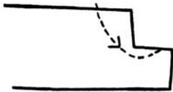
FIG. 24. DIAGRAM SHOWING PIERCING TOO DEEP
