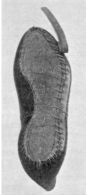
Fig. 51. ANGLE OF WELT LEVEL TO UPPER
