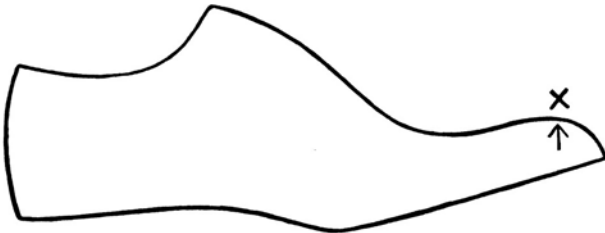
FIG. 38. DIAGRAM SHOWING LAST WITH RESISTANCE POINT AT X
